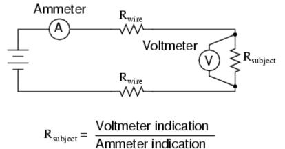
Current is the same at all points in the circuit, because it is a series loop. Because we're only measuring voltage dropped across the subject resistance (and not the wires' resistances), though, the calculated resistance is indicative of the subject component's resistance (R<sub>subject</sub>) alone.
